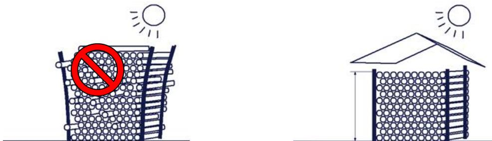
The pallets' side holders should be placed at maximum intervals of 1,5m. The pipes should be supported throughout its length. Pipes of different diameters and thicknesses should be stored separately. If not possible, the ones with bigger diameter and thickness should be placed in the back.
